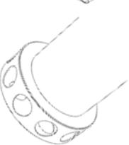
The flat suction strainer is suitable for pumping down to the lowest possible surface. (Not suitable for large volumes and soft ground).
