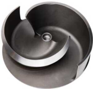
Semi-open impeller Corrosion and abrasion resistant pump impeller made of chrome moly (42CrMo4) alloy.
