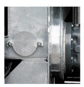
Large inspection covers Easy access to float box, impeller and non-return valve.
