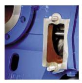
**Easy access points** Allows access to the cylinders, stuffing boxes and other critical areas for easy cleaning and maintenance.
